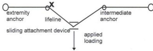
**Figure 4 HLL Tensile Tests to Destruction**
