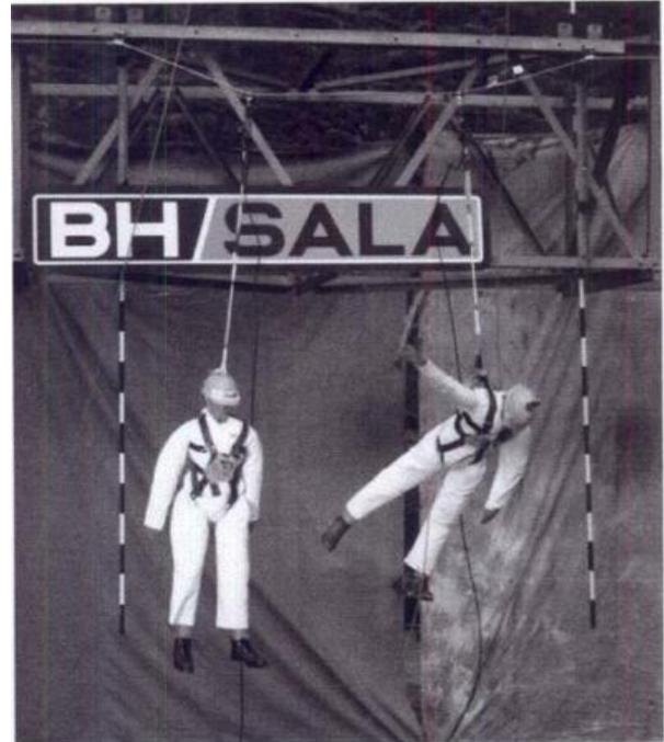
Figure 7: Dummy "George" catches his arm on the HLL on the way down during a "SIMREL"
