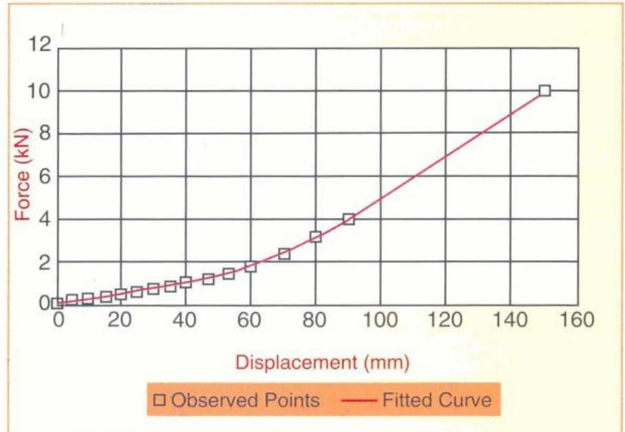
DIAGRAM 1: Elasticity relationship of a typical 7 x 7 construction cable.
